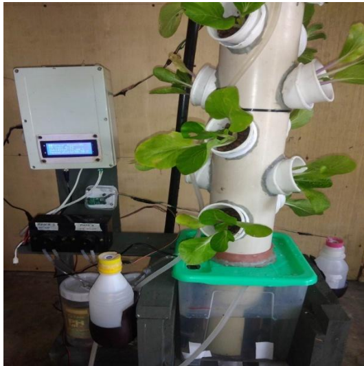
Fig. 9.3.1 Solar powered Vertical Hydroponics System
