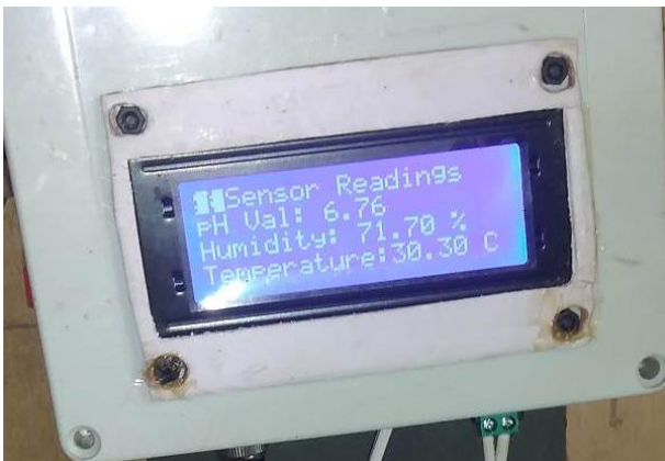
Fig 1.11 PH Level, and Temperature and Humidity Monitoring of prototype Vertical Hydroponic Farm with water level, PH level and humidity-temperature monitoring with automatic watering using IoT.
