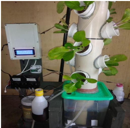
Fig. 1.10 Vertical Hydroponic Farm with water level, PH level and humidity-temperature monitoring with automatic watering using IoT
